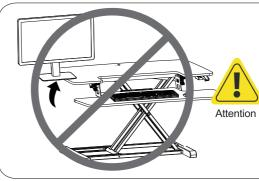
Please make sure all installed equipments are on the table, and not sticking out of the edge, or it may harm or cause damage.
